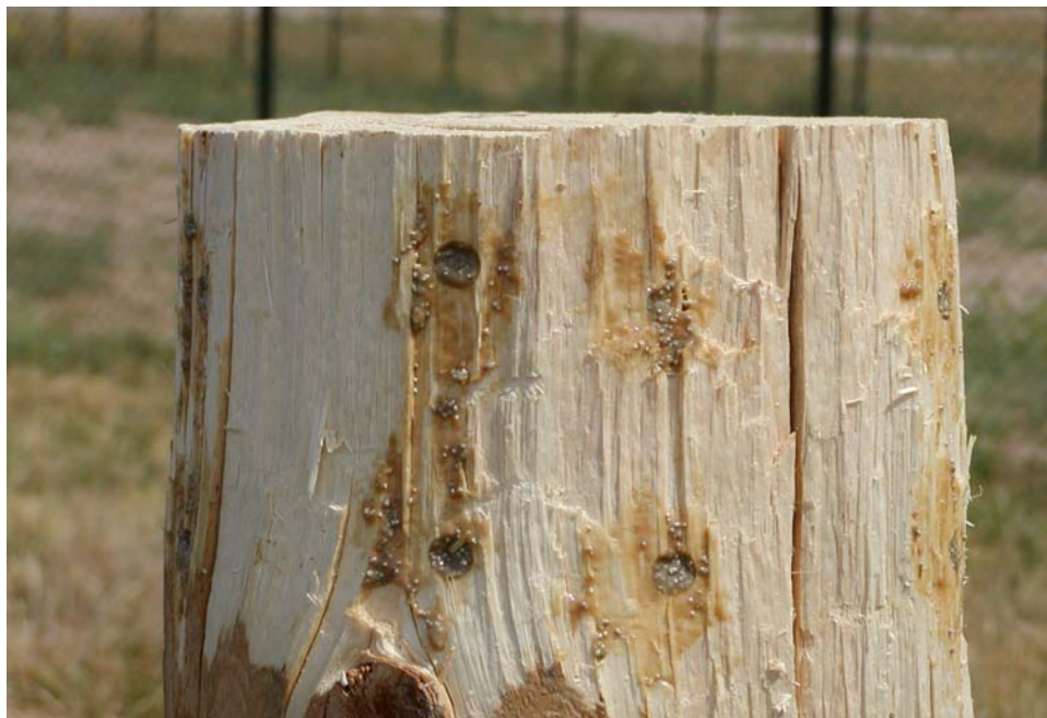
Figure 2: IStop-CC™ Sniff ‘N’ Stop deterrent, plug treatment. Each pole was perforated every 7.6 cm around the circumference of the pole section. Holes were filled with the product using a hand trowel.
