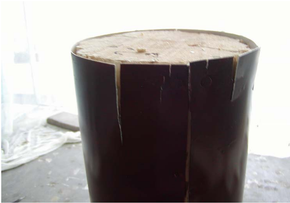
Figure 4: Painted PVC sheeting. This is the same type of sheet material the epoxy resin was applied to. Material was painted to mimic the epoxy treated wrap poles.
